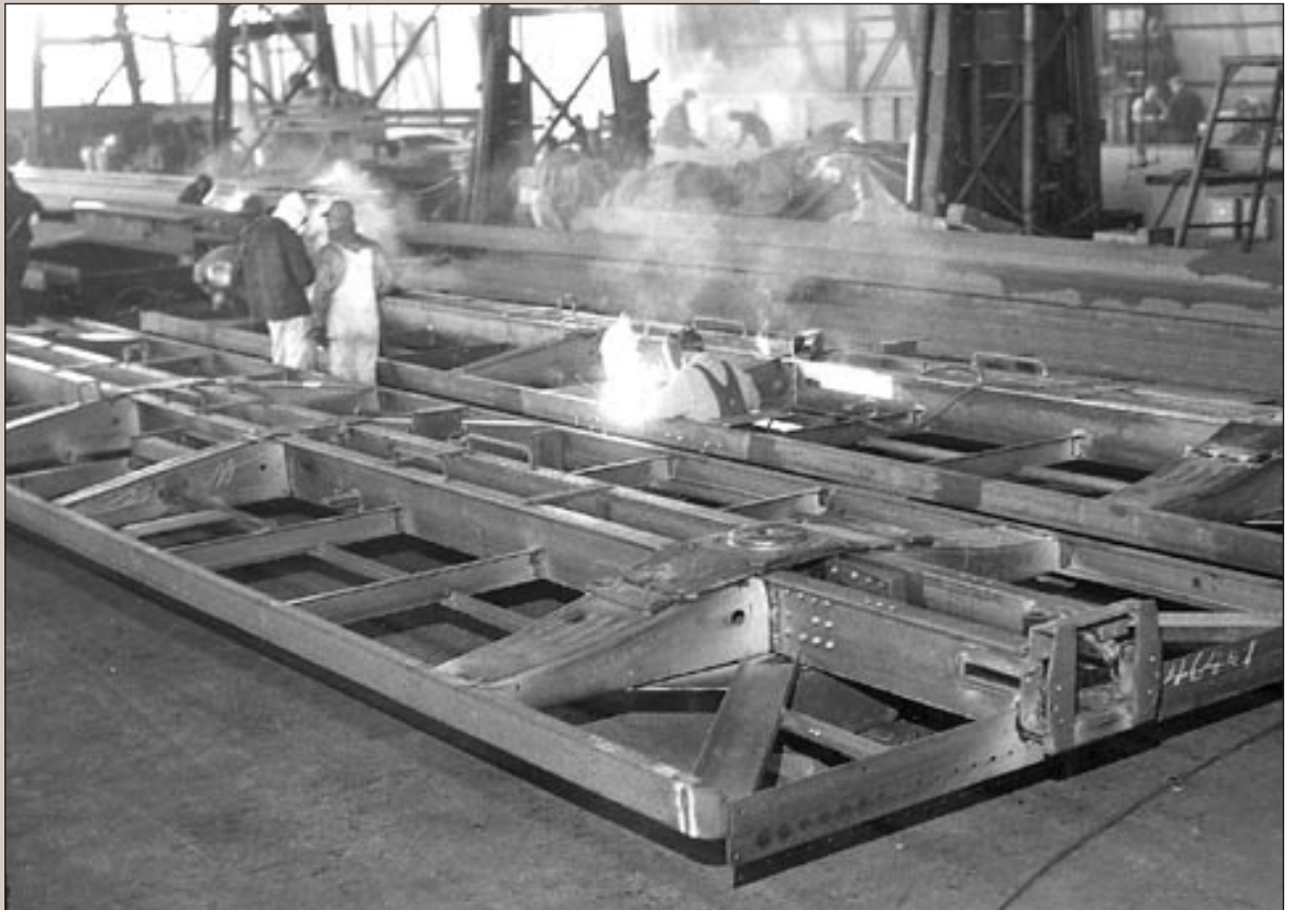
Southern Pacific Railroad started Gunderson in the railcar building business in 1958 with the first order of these boxcar underframes.
