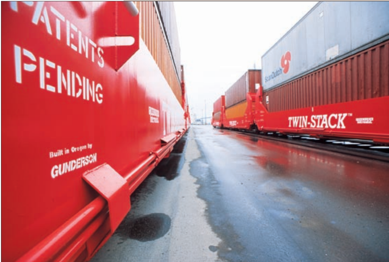
Twin-Stack was the first of a long series of double stack cars marketed by Greenbrier and built at Gunderson.
