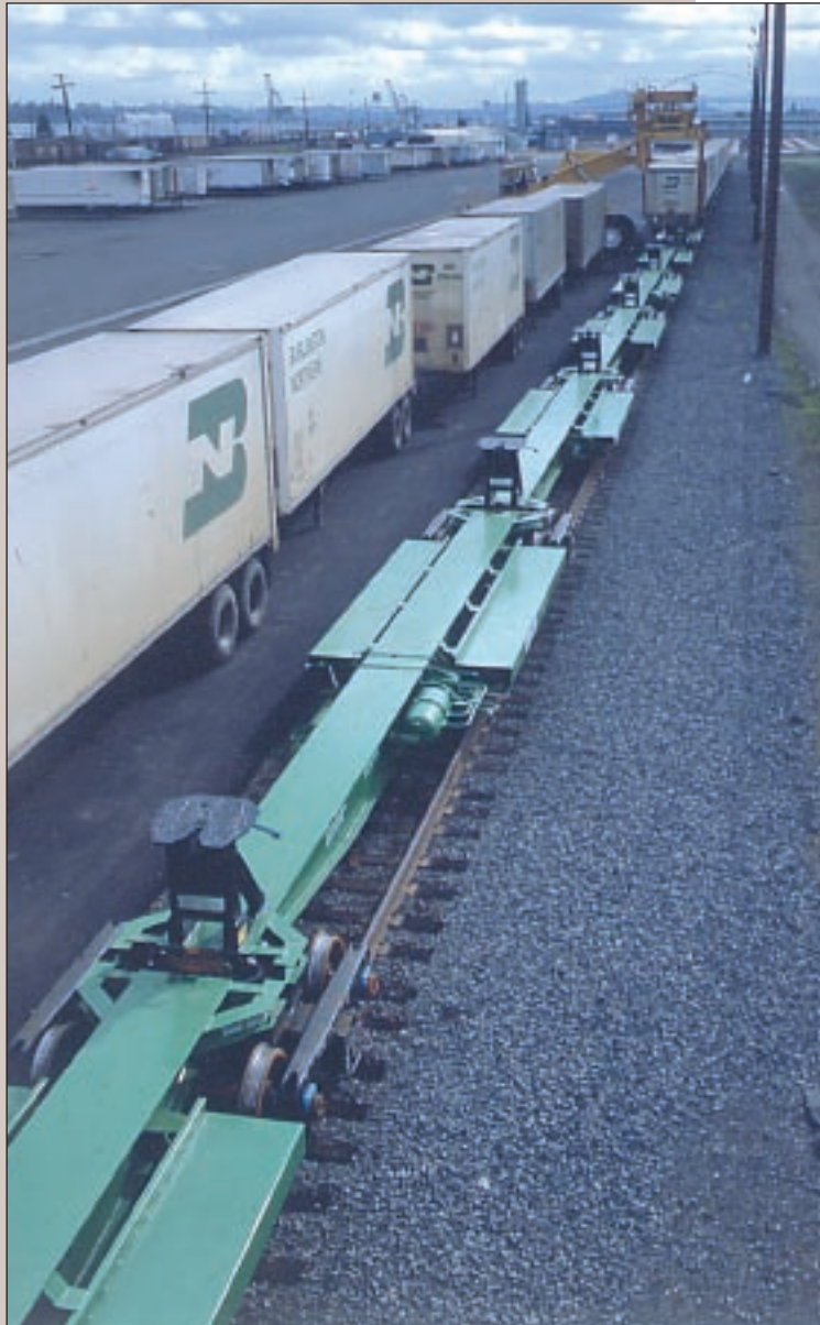
A very light weight articulated car for carrying highway trailers, developed by Santa Fe railroad in the 1970s, was licensed to ITEL Corporation under the name "Impack" and built by the plant during FMC's ownership.
